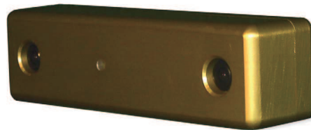
Figure 2.6: Stereo vision camera attached to Gryphon
