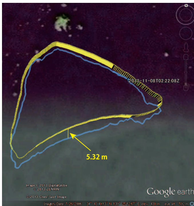
Figure 6.20: GPS data comparison between Gryphon' GPS (yellow) and a hand GPS (blue)
