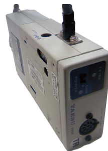
Figure 2.13: Yaesu modem for RTK
