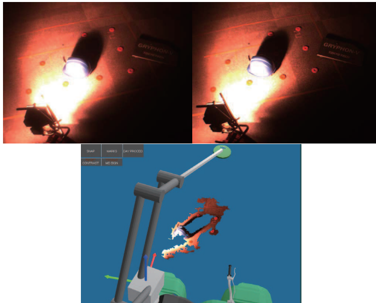
Figure 6.6: Effect of strong light contrast in the map calculation. Camera's left-right pair images (top) and calculated depth map displayed in the user interface (bottom)
