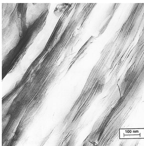
Fig. 1.3 Bright-field TEM of poly(3-bromostyrene)-F12 (dodecylammonium-exchanged fluorohectorite) [10]
