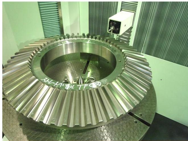
Fig. 5.8 Measurement of gear member
