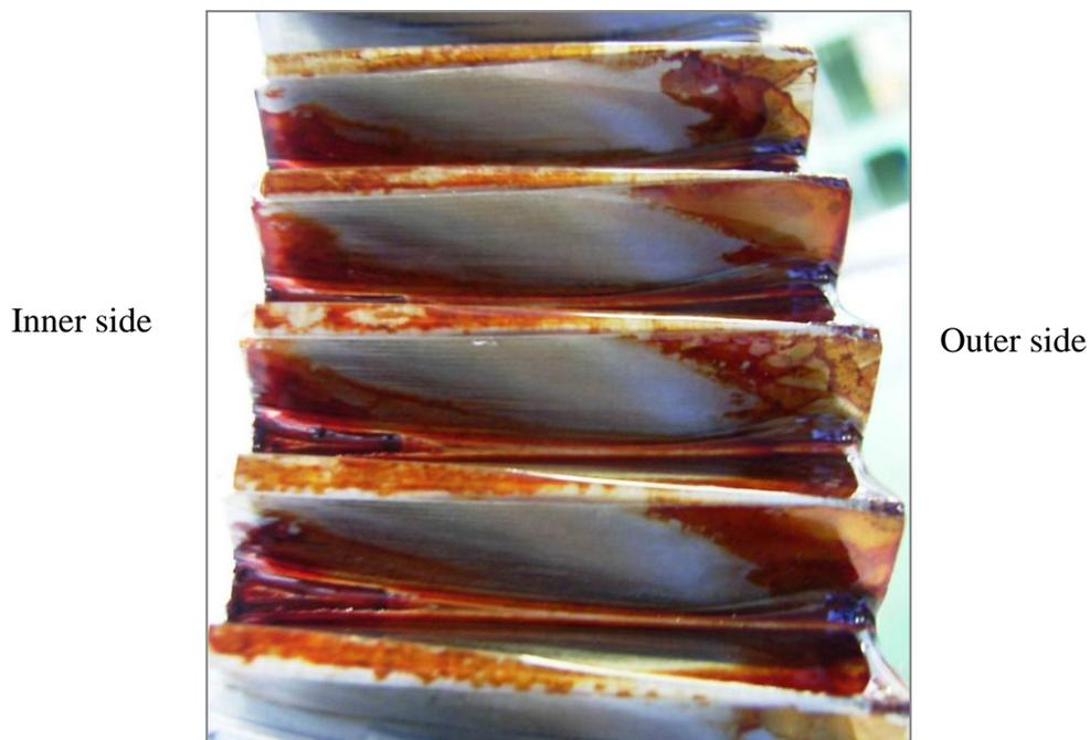
Fig. 5.29 Tooth contact patterns after running test
