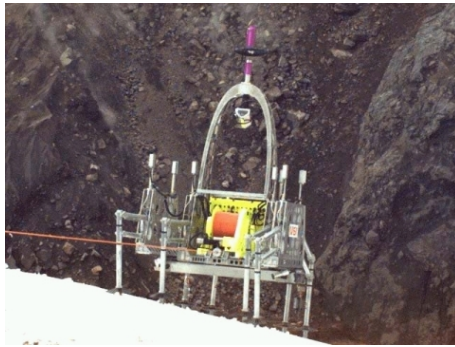
(a) Dante II using tether-based rappelling locomotion[26].
