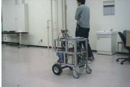
Figure 1.5: Escort robot using camera and light emitting device, developed by Ohya and Nagumo[16]
