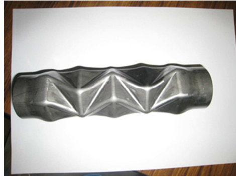
Fig. 7.2 Sample of Origami Side Member Manufactured by Hydro-forming.
