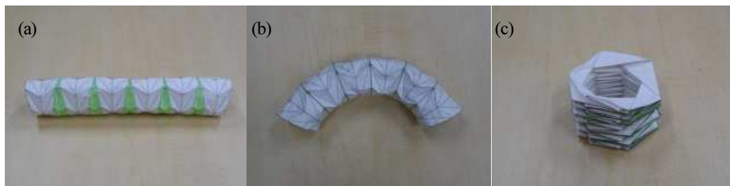
Fig. 6.12 Flat-Foldable Meandering Cylinders Based on Folding with Six Fold Lines without Cutting-Off: (a) Straight cylinder if perfectly inflated; (b): Meandering cylinder. Green parts are glued; (c) : Folded cylinder.
