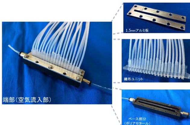
Fig. 4 Specification of each part
