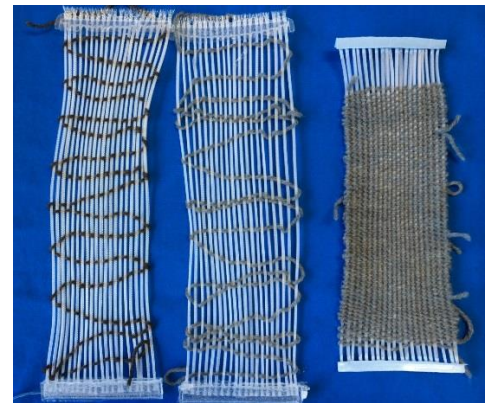
Fig. 7 Active textile woven by semi-automatic weaving machine with different pitch
