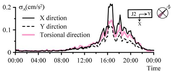
Figure 12. Standard deviation of top floor acceleration  $\sigma_A$
