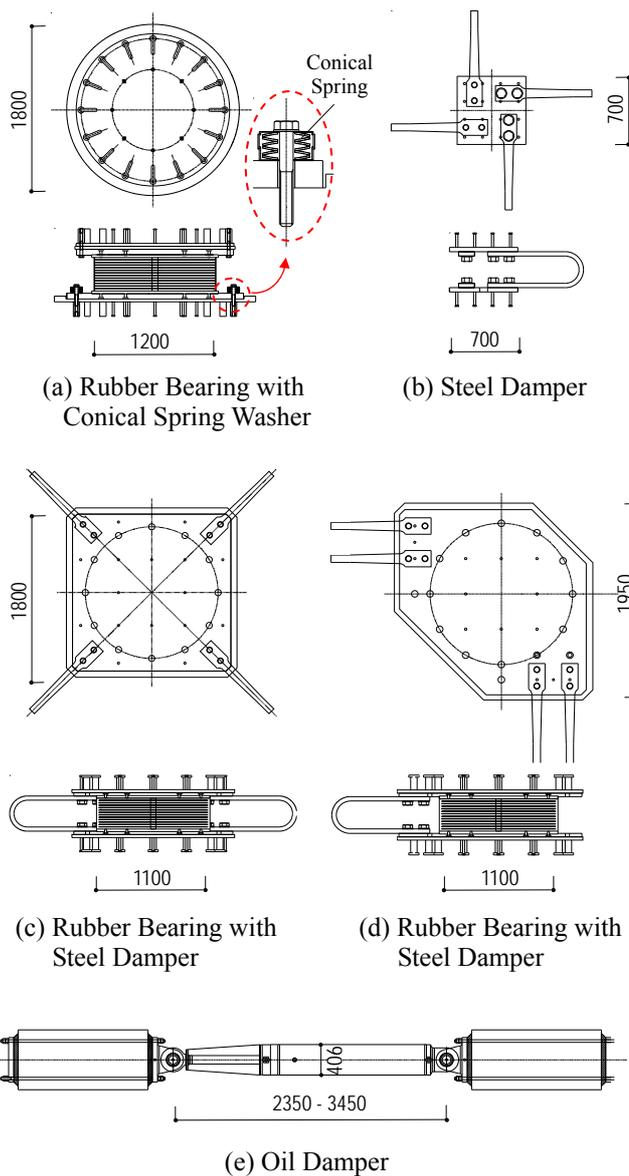
Figure 4. Rubber Bearing and Damper (unit: mm)
