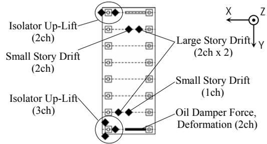
Figure 6. Configuration of displacement transducers at isolation floor
