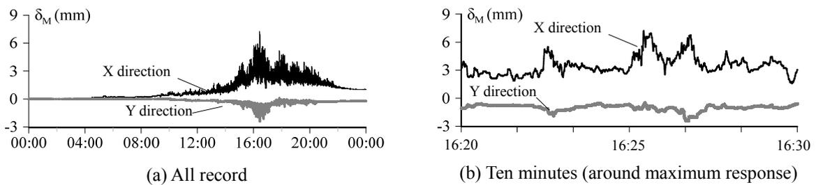
Figure 18. Deformation of seismic isolation layer  $\delta_M$
