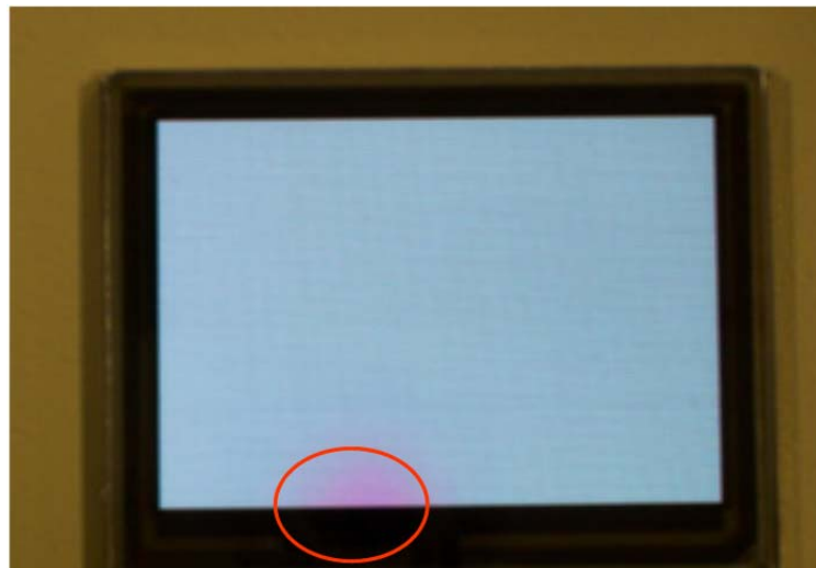
Fig. 94 Colored non-uniformity region caused by shadow-mask process
