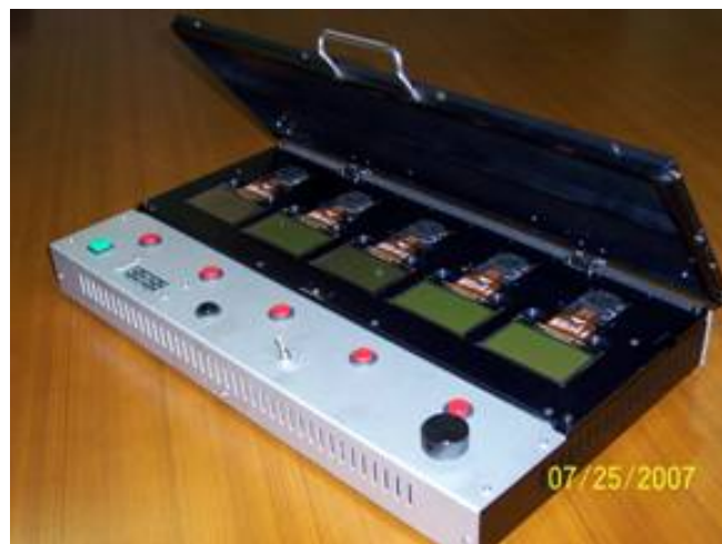
Fig. 124 Equipment used for the external mura compensation
