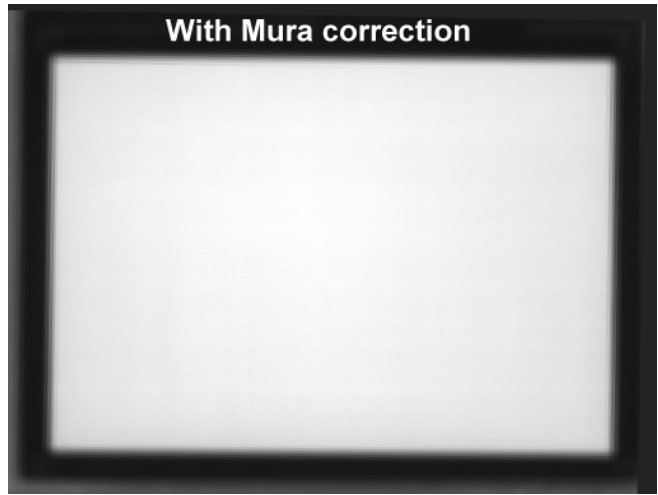
Fig. 127 Display uniformity of LTPS AMOLED display with external compensation
