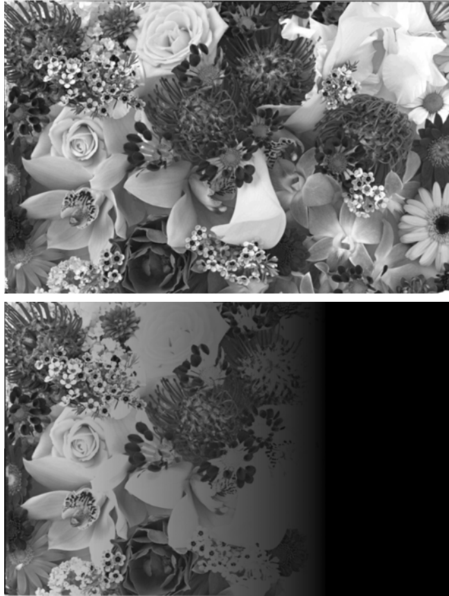
Fig. 56 Displays with small voltage drop and large voltage drop
