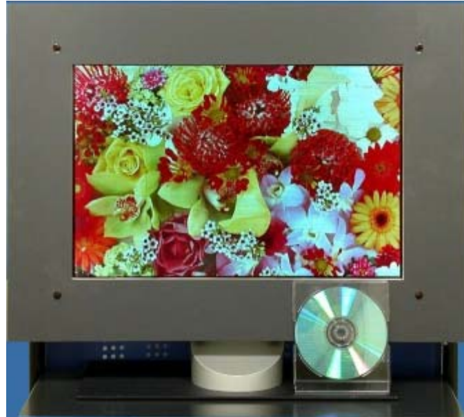
Fig. 55 20.0" world's largest (at the time) active-matrix OLED display driven by amorphous silicon TFT backplane
