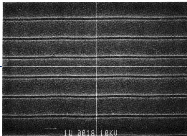
Fig.3.38(d) Surface roughness of the land surface of the polycarbonate substrate (MO sputtered surface)
