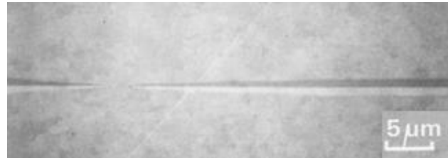
(a) Vertical load F=0.47\text{mN}
