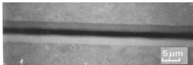
Fig. 3.12 Sub-micron order depth V-shaped groove by Thickness Control Cutting Method
