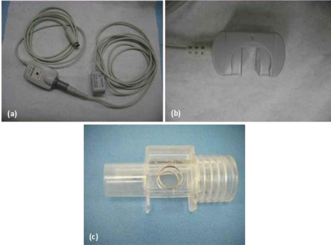
Fig. 2.15. Parts of capnograph Capnosafe: (a) IR sensor of \text{CO}_2 and processing module. (b) Detail view of the sensor. (c) Airway adapter.
