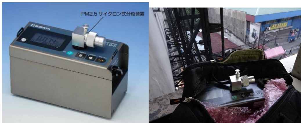
Figure 4.1. SIBATA PM 2.5 Cyclone for LD-5 equipment
