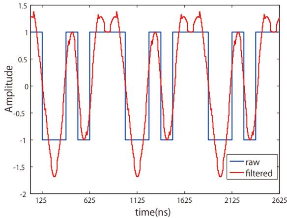
Fig. 7 Band-limited M-sequence code by roll-off filter
