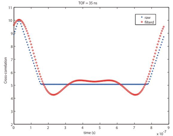
Fig. 8 Cross-correlation function with band-limited signals (TOF = 35 ns)
