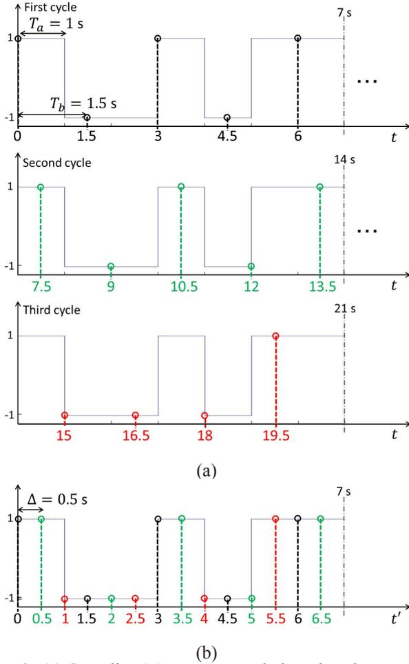
Fig. 3 (a) Sampling M-sequence code based on heterogeneous clock system ( $n = 3$ ,  $T_a : T_b = 2 : 3$ ) (b) Reconstructed M-sequence code
