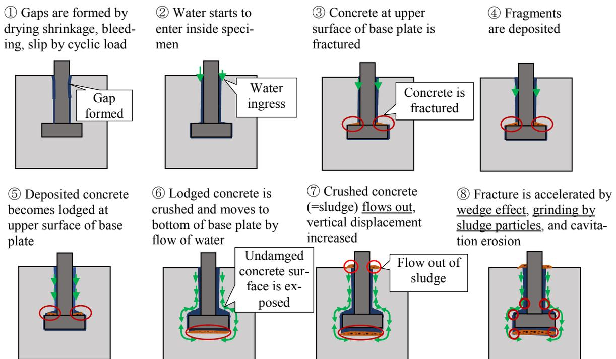
Fig. 15 Breakdown development mechanism around anchor.
