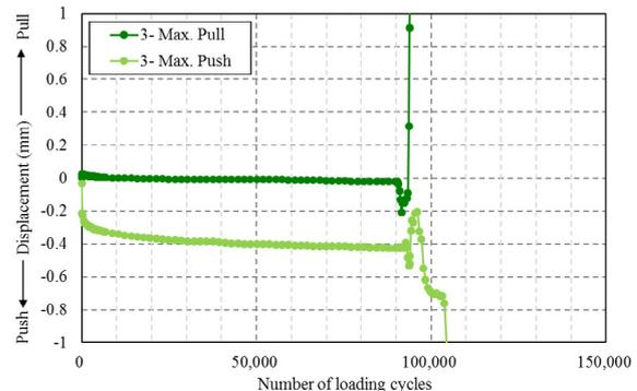
Fig. 9 Characteristic displacement before pull acceleration (Case 3 example).
