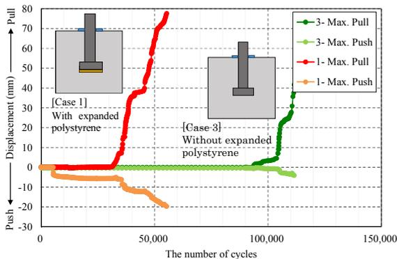
Fig. 8 Relationship between reduction of interfacial bond and accompanying reduction of anchorage performance.
