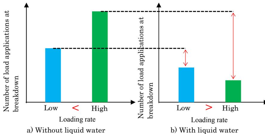
Fig. 13 Influence of loading rate in presence of liquid water.
