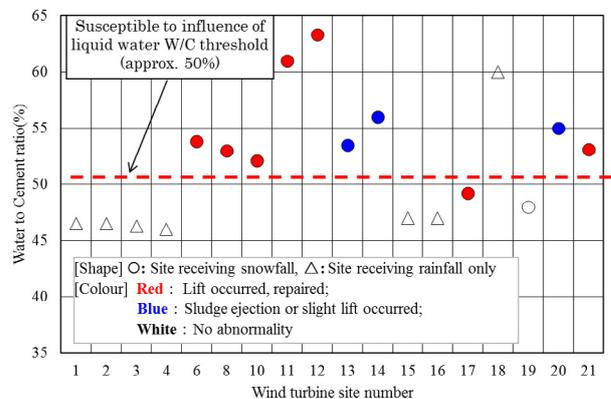
Fig. 16 Relationship between lifting of tower, W/C, and environmental conditions.
