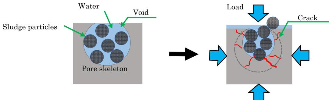
Pore is fulfilled by water with some sludge particle.
