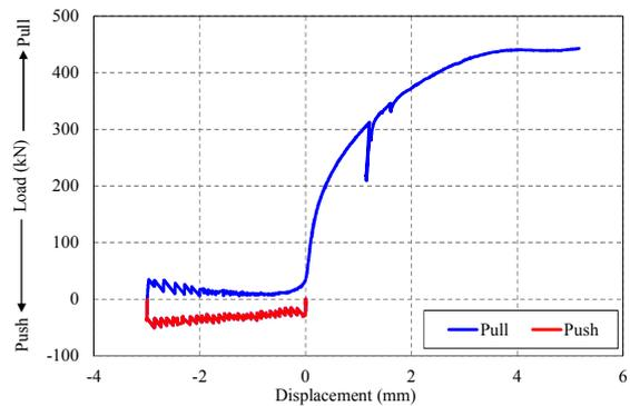
Fig. 5 Static push and pull test results.
