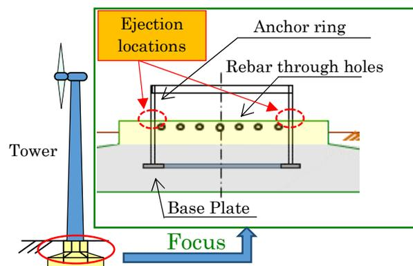
Fig. 1 Anchorage zone and sludge ejection locations.
