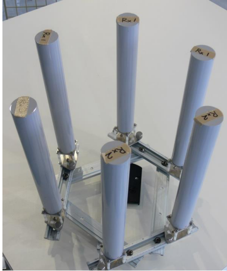
Figure 5.6 Photo of the antenna orientation at Tx for multi-link measurement (6-elements configuration).
