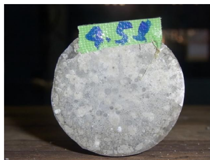
(b) Specimen B Water ratio 18.0 % (4.5 ℓ/25 kg)
