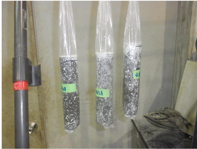
Fig. 2-17 Bleeding test of mortar
