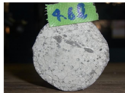
(c) Specimen C Water ratio 18.4 % (4.6 ℓ/25 kg)
