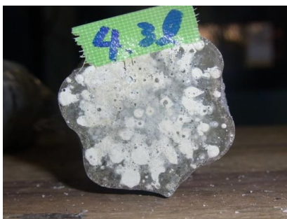
(a) Specimen A Water ratio 17.2 % (4.3 ℓ/25 kg)
