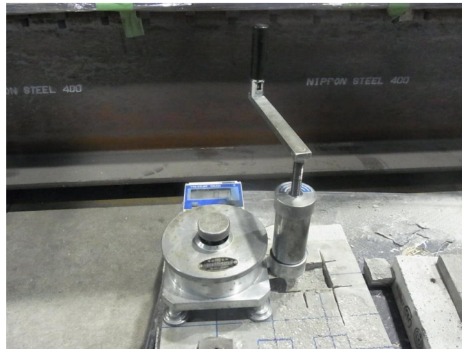
Fig. 2-21 Test equipment for bonding test
