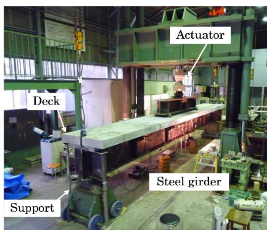
Fig. 3-8 Specimen under loading test
