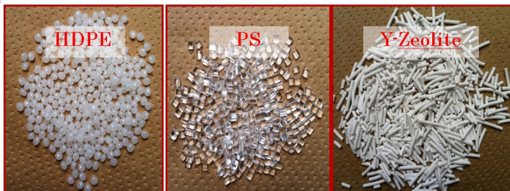
Fig. 2.1. The photographs of feedstock samples (HDPE and PS) and Y-Zeolite catalyst.
