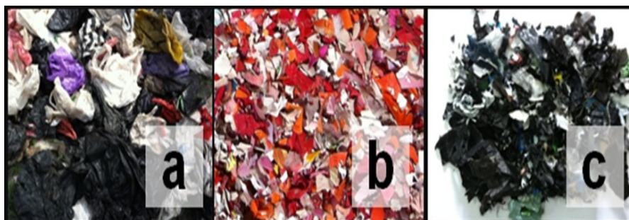
Fig. 4.2. The feedstock used in the experiments : a) PE bag 1, b) HDPE waste dan c) PE bag 2
