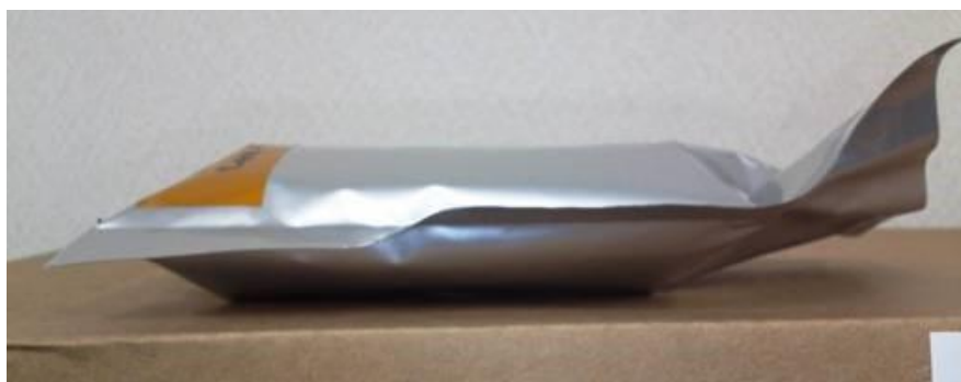
Figure 53 Typical picture of High Voltage swelled Laminate cell.
