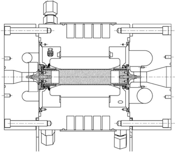
Fig.2 Cross Section of Gas Turbine Power Generator
