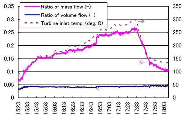
Fig.12 Trend of Leak Flow Ratio (No.20)
