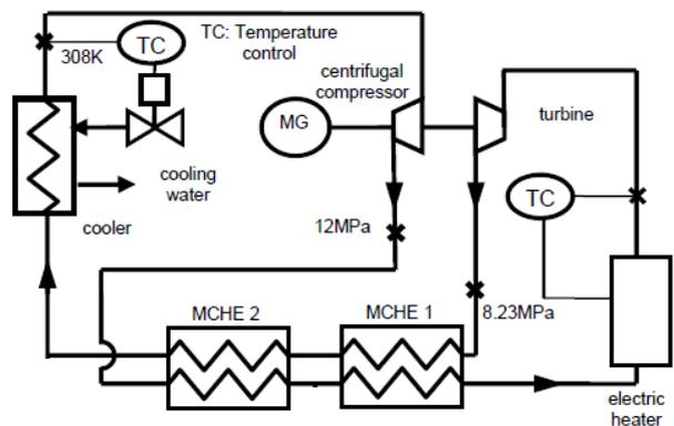
Fig.1 Flow Diagram of CO<sub>2</sub> Loop for Brayton Cycle
