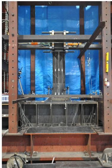
Photo 4.1 Monotonic bending shear test
