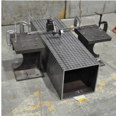
Photo 3.4 Measurement test of initial deflection
