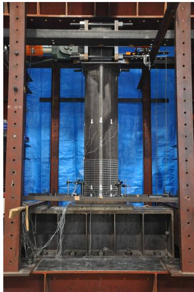
Photo 5.1 Cyclic bending shear test
