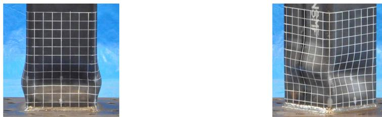
(a) Angle of applied force 0 deg.      (b) Angle of applied force 45 deg.
