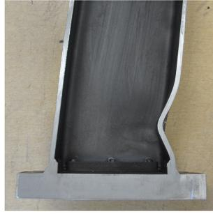
Cold roll formed BCR295 200×200×8 Shear span ratio 6 Angle of applied force 0 deg.
