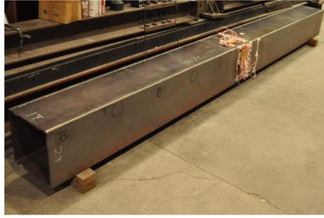
Photo 3.3 Measurement test of residual stress for long specimen
