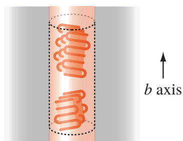
Figure 1.4. Schematic illustration showing the crystal orientation of PE homopolymers confined in AAO nanopores 19 .
