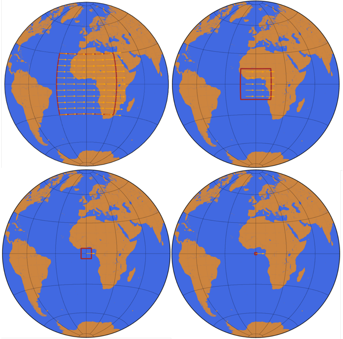
Fig. C.1 Straight motion of ideal plates with a different plate size. The size: [top, left] Large: 60^\circ \times 60^\circ ; [top, right] Small: 30^\circ \times 30^\circ ; [bottom, left] Tiny: 10^\circ \times 10^\circ ; [bottom, right] Micro: 2^\circ \times 2^\circ . All the plate has the same Euler pole at the North Pole and orange vectors represents the induced eastward motion.
