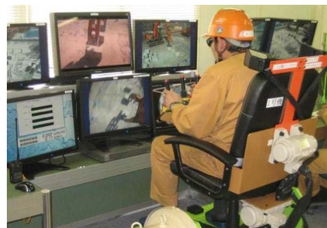
Fig.1.12 Obayashi remote controller for the heavy machinery (Ref.[31])
