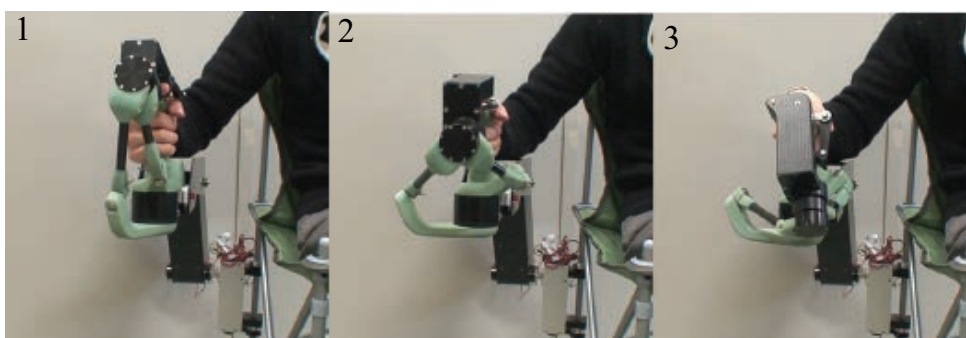
Fig.3.35 Workrange around Pitch axis on the posture controller
