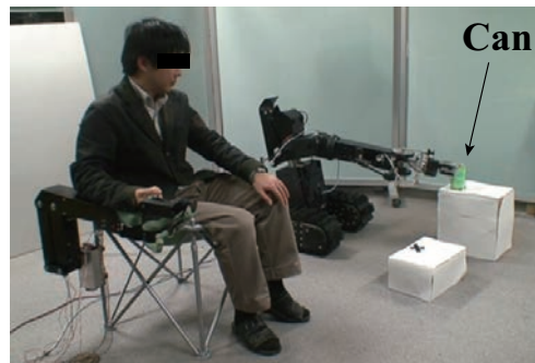
Fig.4.35 Experiment to make the Helios IX grab the can with the weight
