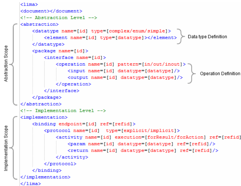
Figure 18. The structure of the LIMA description.
