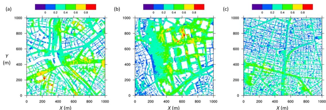
**Figure 6.12** Gust index distribution at 2 m height for the 1,000 m  $\times$  1,000 m of the (a) commercial land, (b) skyscrapers and (c) residential area by using the proposed definition.
