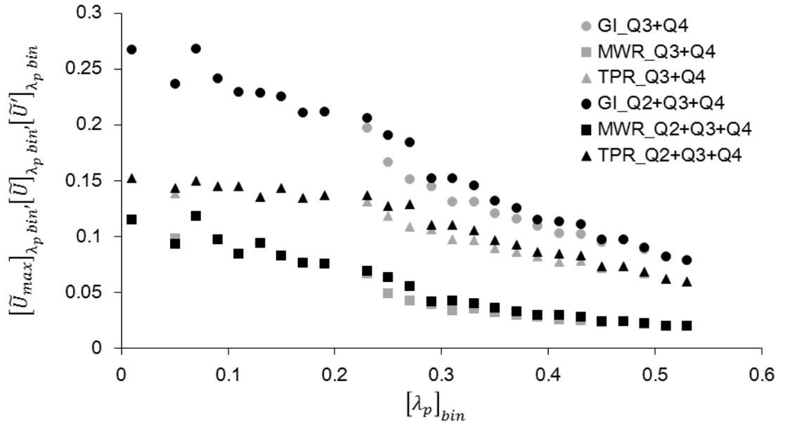
**Figure 7.7** The spatial and bin average of the  $480 \times 480 \text{ m}^2$  patches for the gust index,  $[\tilde{U}_{max}]_{\lambda_p bin}$ , mean wind speed ratio,  $[\tilde{U}]_{\lambda_p bin}$ , and turbulent part ratio,  $[\tilde{U}']_{\lambda_p bin}$ , versus the plan area index,  $[\lambda_p]_{bin}$ , at 2 m for the last three quarters from the domain inlet (Q2 + Q3 + Q4) and the latter of the half domain (Q3 + Q4).
