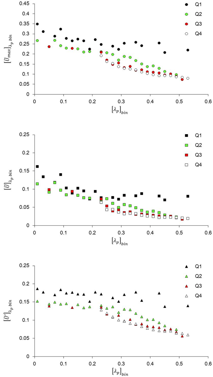
**Figure 7.4** The spatial and bin average of the  $480 \times 480 \text{ m}^2$  patches for the gust index,  $[\tilde{U}_{max}]_{\lambda_p bin}$ , mean wind speed ratio  $[\tilde{U}]_{\lambda_p bin}$ , and turbulent part ratio,  $[\tilde{U}']_{\lambda_p bin}$  versus the plan area index,  $[\lambda_p]_{bin}$ , at 2 m for the whole domain divided into four quarter in the streamwise direction.
