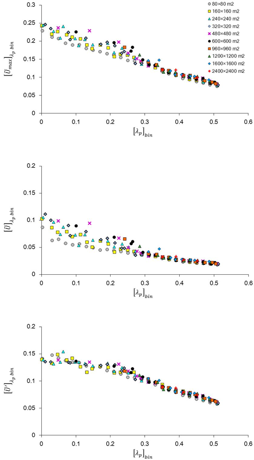
**Figure 7.1** The bin analysis of the spatial average of the different patch sizes of the (a) gust index,  $[\tilde{U}_{max}]_{\lambda_p bin}$ , (b) mean wind speed ratio,  $[\tilde{U}]_{\lambda_p bin}$ , and (c) turbulent part ratio,  $[\tilde{U}']_{\lambda_p bin}$ , versus the plan area index,  $[\lambda_p]_{bin}$ , at 2 m height for the latter half of the simulation domain.
