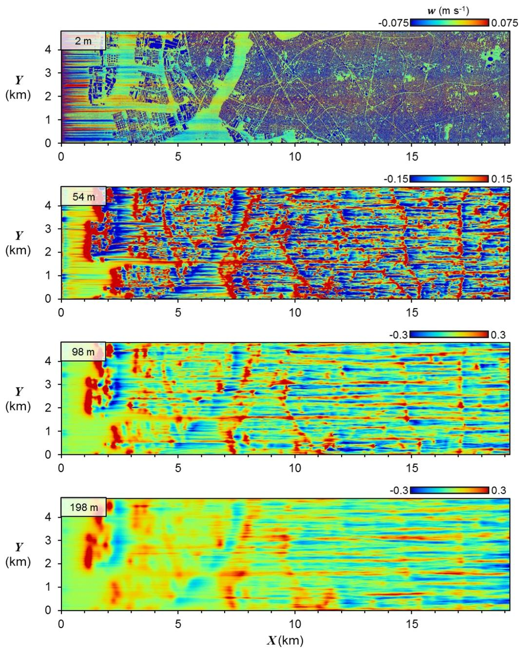
**Figure 6.4** Horizontal distribution ( $xy$ -plan) of the mean wind velocity ( $w$ -component) at 2, 54, 98 and 198 m height.
