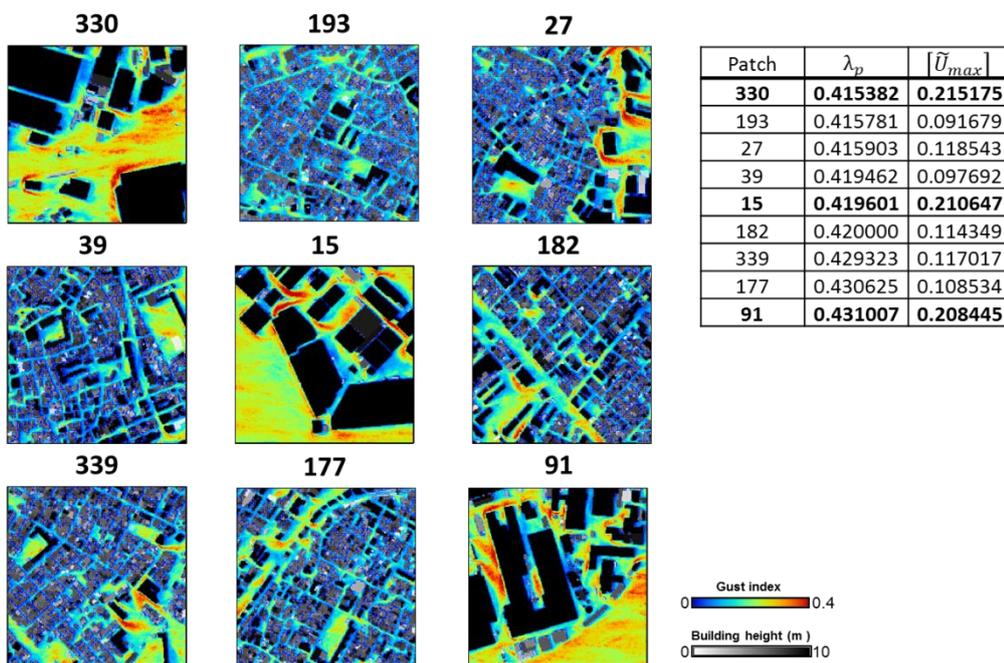
**Figure 7.6** Selected  $480 \times 480 \text{ m}^2$  patches of Fig. 7.5 and its corresponding plan area index,  $\lambda_p$  and gust index,  $[\tilde{U}_{max}]$ . Isolated scatter plot (Patch 15, 91 and 330) and closed to linear trendline (others).
