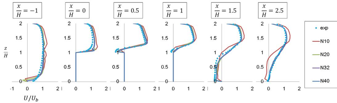
**Figure 4.2** Vertical profile of the average wind speed,  $U$ , normalized to the bulk inflow cross-section average wind speed,  $U_b$ . Experiment data shown by the dotted line. Each profile represents the position mentioned in Fig. 4.1.
