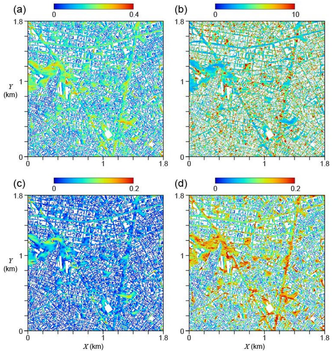
**Figure 6.14** Magnified view overlain with the building height of the (a) gust index,  $\tilde{U}_{max}$ , (c) mean wind ratio,  $\tilde{U}$ , (d) turbulent part ratio,  $\tilde{U}'$ , from Fig. 6.13 and (b) the spatial distribution of the conventional gust factor,  $G$ .
