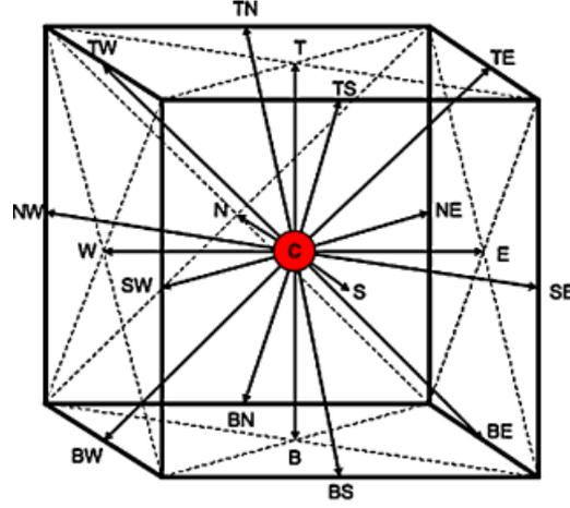
**Figure 3.2** The arrows represent the directions of the fluid populations (i.e., a set of 18 discrete velocities including one null vector corresponding to particles at rest) according to the D3Q19 scheme [Bernaschi et al. \(2010\)](#).
