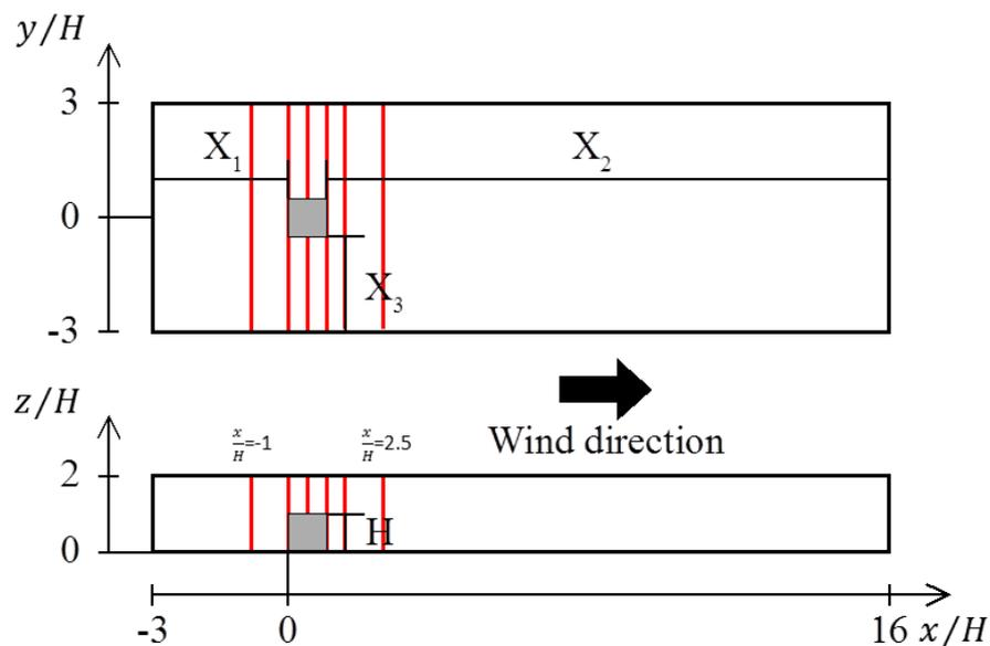
**Figure 4.1** Domain setting for the validation simulation. Red lines show each measurement location ( $x/H = -1, 0, 0.5, 1, 1.5, 2.5$ ).
