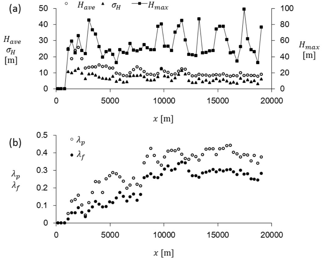
**Figure 5.1** Geometry parameter of the simulation domain. (a) Maximum building height,  $H_{max}$ , average building height,  $H_{ave}$  and its standard deviation  $\sigma_H$ . (b) The plan area index,  $\lambda_p$  and frontal area index,  $\lambda_f$ .
