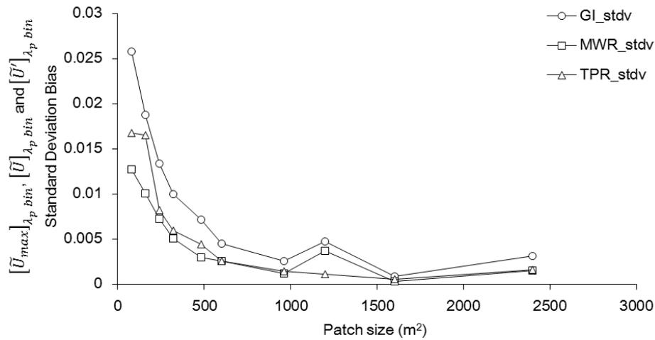
**Figure 7.2** Standard deviation bias analysis of the different patch sizes ( $\text{m}^2$ ) from the gust index,  $[\tilde{U}_{max}]_{\lambda_p \text{ bin}}$ , mean wind speed ratio,  $[\tilde{U}]_{\lambda_p \text{ bin}}$ , and turbulent part ratio,  $[\tilde{U}']_{\lambda_p \text{ bin}}$ .
