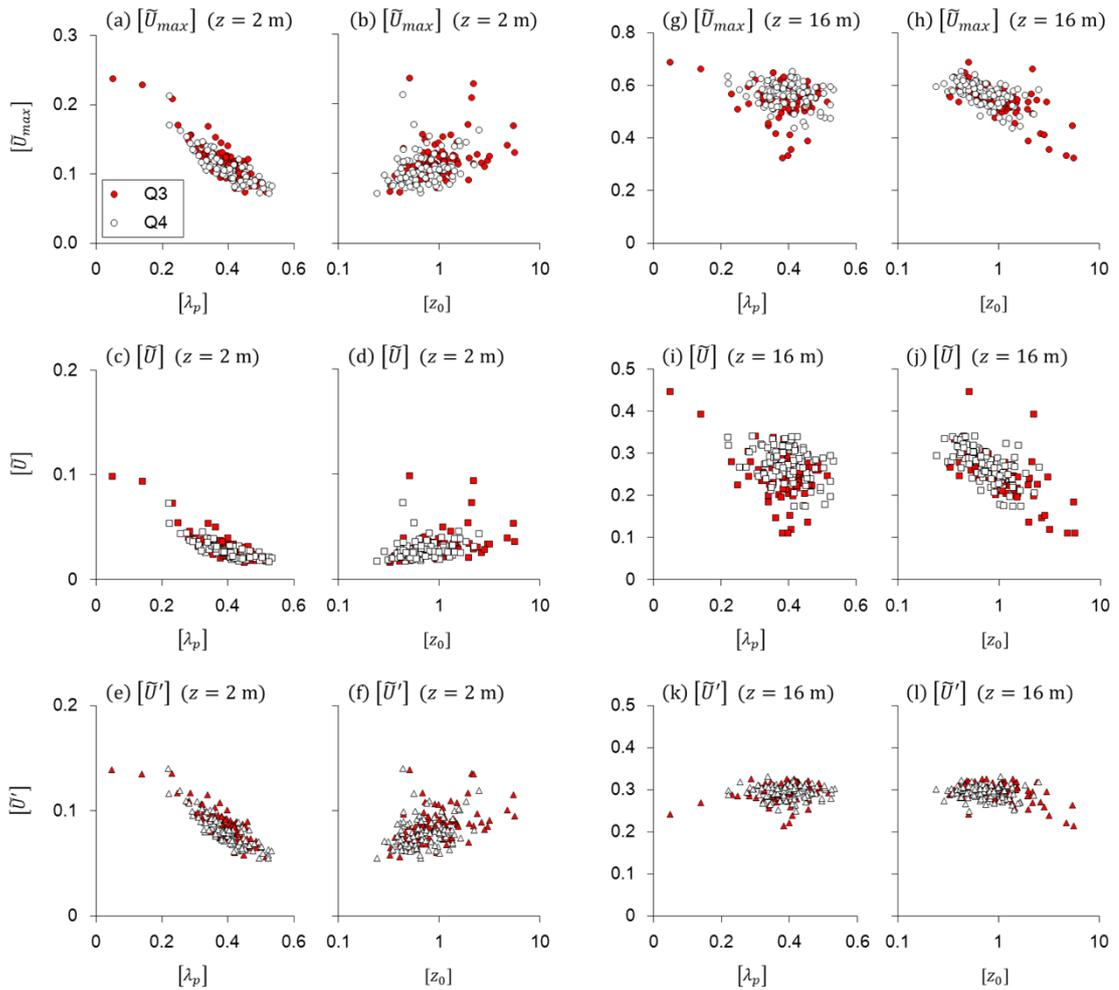
**Figure 7.10** The gust index,  $[\tilde{U}_{max}]$ , mean wind speed ratio,  $[\tilde{U}]$ , and turbulent part ratio,  $[\tilde{U}']$ , versus the plan area index,  $[\lambda_p]$ , and the roughness length,  $[z_0]$  in the  $480 \times 480 \text{ m}^2$  patches at a height of 2 and 16 m for the latter half of the domain (Q3 + Q4).
