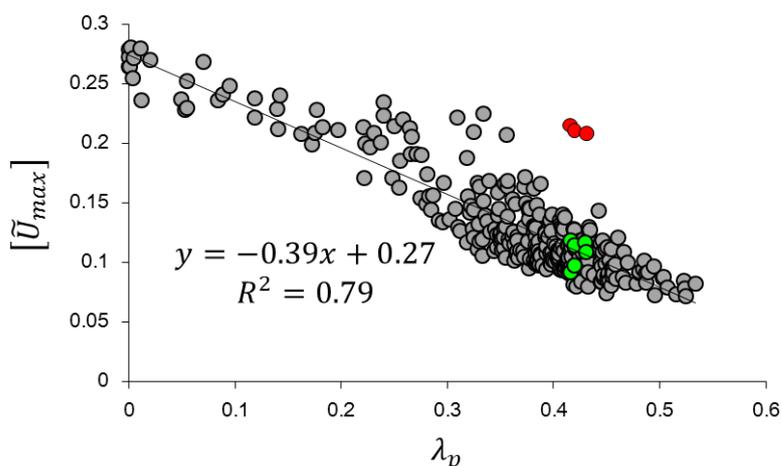
**Figure 7.5** The spatial average of the  $480 \times 480 \text{ m}^2$  patches for the gust index,  $[\tilde{U}_{max}]$  versus the plan area index,  $\lambda_p$ , at 2 m for the last three quarters (Q2+Q3+Q4). Chosen isolated scatter plots (red circle) and closed to linear trendline (green circle) were  $0.415 < \lambda_p < 0.432$ .
