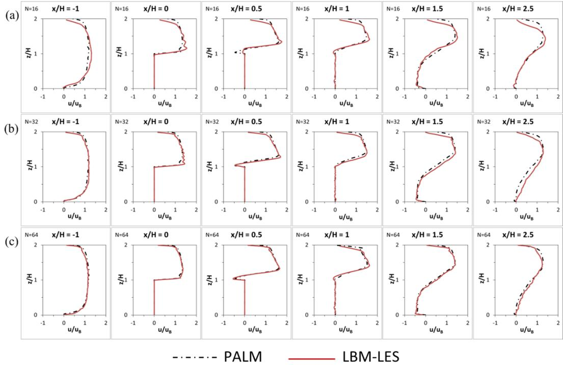
**Figure 4.4** Comparison between the PALM and LBM-LES vertical profile of  $U/U_b$ . Domain resolution of (a) 3 m ( $N = 16$ ), (b) 1.5 m ( $N = 32$ ) and (c) 0.75 m ( $N = 64$ ) is homogeneous in all direction ( $dx=dy=dz$ ).
