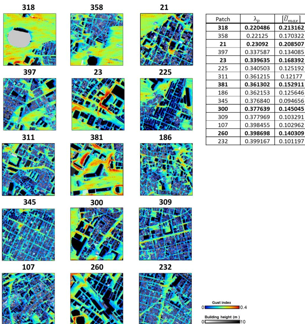
**Figure 7.9** Selected  $480 \times 480 \text{ m}^2$  patches of Fig. 7.8 and its corresponding plan area index,  $\lambda_p$  and gust index,  $[\tilde{U}_{max}]$ . Isolated scatter plot (Patch 21, 23, 260, 300, 318 and 381) and closed to linear trendline (others).
