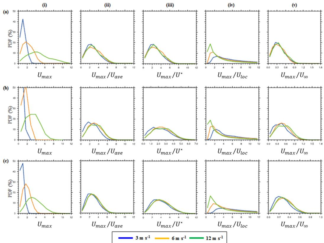
**Figure 4.5** Probability density distribution of the (i) maximum wind speed,  $U_{max}$  and for four different definitions of the gust index, (ii)  $U_{max}/U_{ave}$ , (iii)  $U_{max}/U^*$ , (iv)  $U_{max}/U_{loc}$ , (v)  $U_{max}/U_{\infty}$  for the (a) commercial land (b) skyscrapers (c) residential area. Different line colours show the change in the input wind speed.
