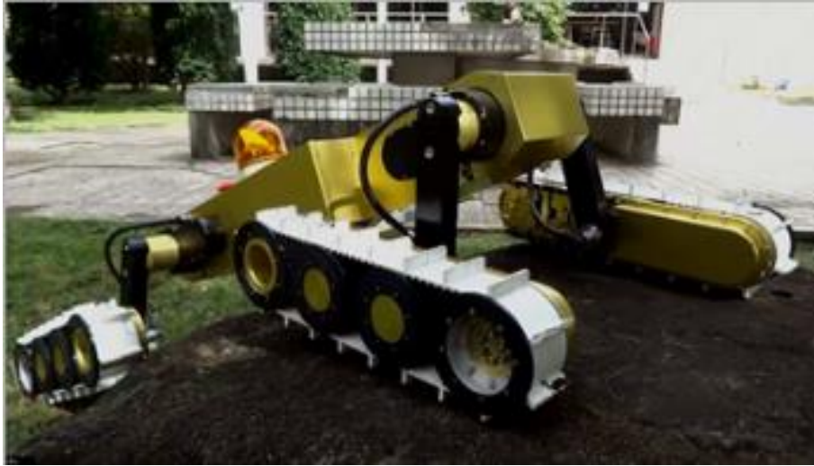
Figure 5-9 Hill climbing test for transformable exploring robot
