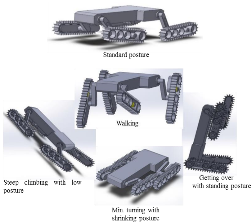
Figure 5-7 Pilot model of transformable exploring robot
