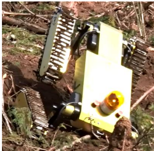
Figure 5-10 Control failure in slope climbing
