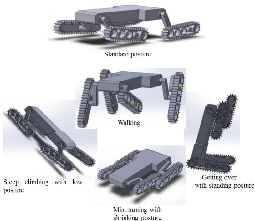
Figure 5-7 Pilot model of transformable exploring robot
