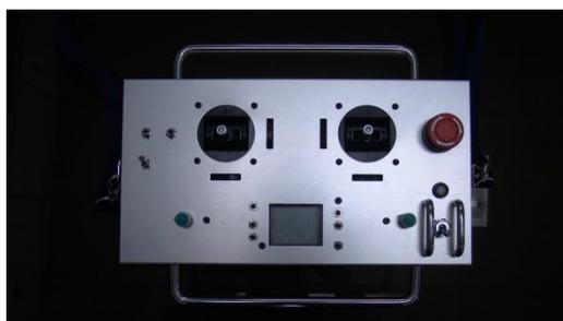
Figure 6-15 Control box for Kenage ver.1
