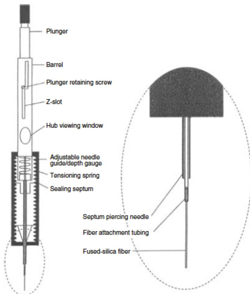
**Figure 2-3.** Schematic diagram of SPME device (Adapted from Gyorgy Vas and Karoly Vekey *J.Mass Spectrom.* 2004;39:233-254 )
