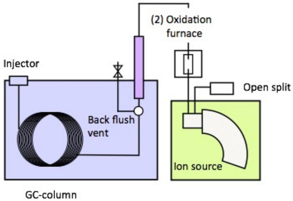
**Figure 2-1.** Schematic diagram of GC-C-IRMS system
