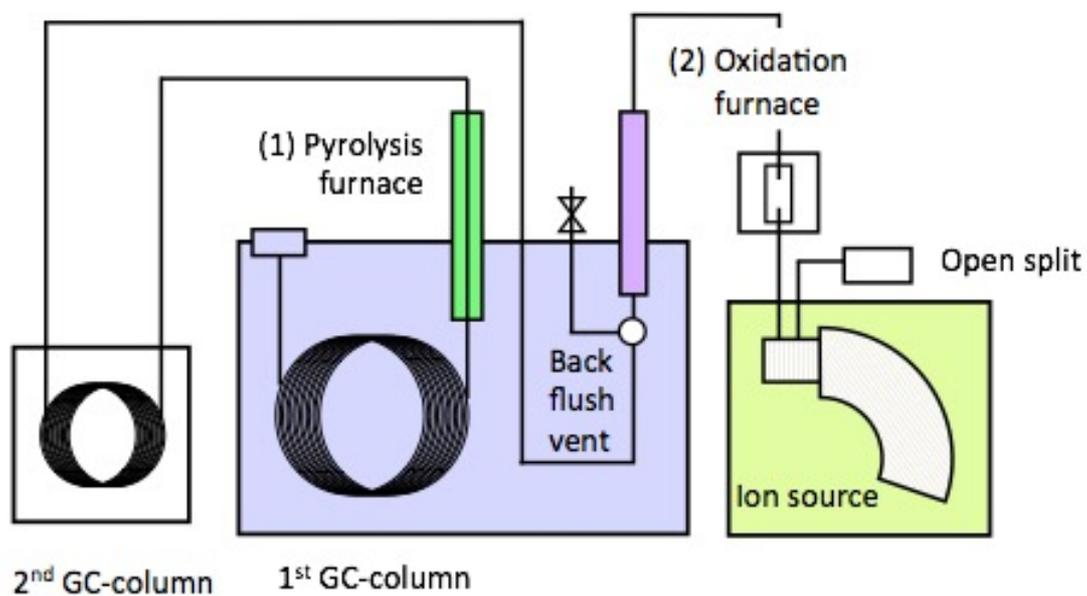
**Figure 2-2.** Schematic diagram of GC-Py-GC-C-IRMS
