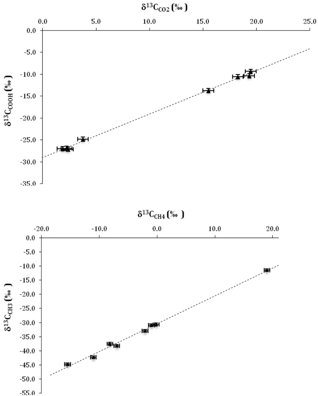
**Figure 2-4.** Correlation curves for certified intramolecular  $\delta^{13}\text{C}$  values ( $\delta^{13}\text{C}_{\text{COOH}}$  and  $\delta^{13}\text{C}_{\text{CH}_3}$ ) and those measured using the online method examined in this study ( $\delta^{13}\text{C}_{\text{CO}_2}$  and  $\delta^{13}\text{C}_{\text{CH}_4}$ ). The dotted line shows best linear fitting (see text for equations and  $R^2$ ).
