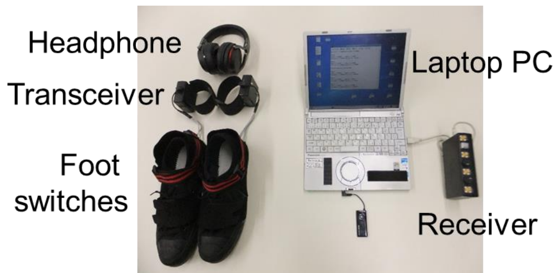
Fig. 4-2-1 Gait training system. Foot switches were attached to the soles of shoes. When the foot is in contact with the ground, the switch is on. The foot contact information is transmitted to laptop PC via wireless communication.
