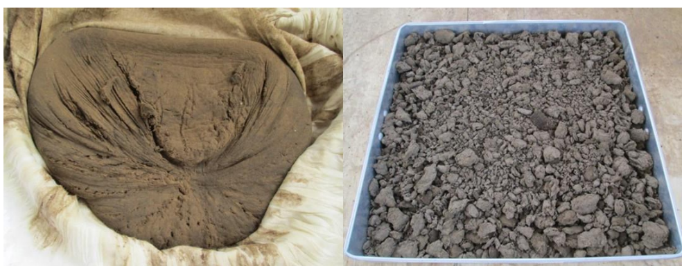
Figure 2-9 Hydrothermally treated paper sludge after dewatering test (left) and naturally dried (right)
