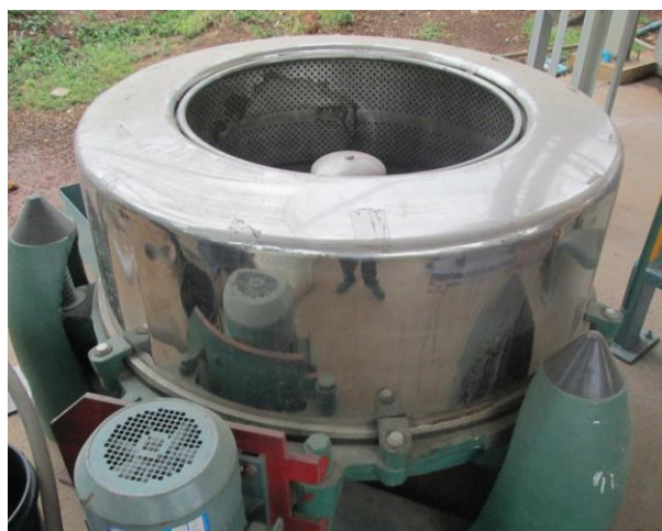
Figure 2-6 1.5 kW centrifugal decanter (Courtesy of SCG)
