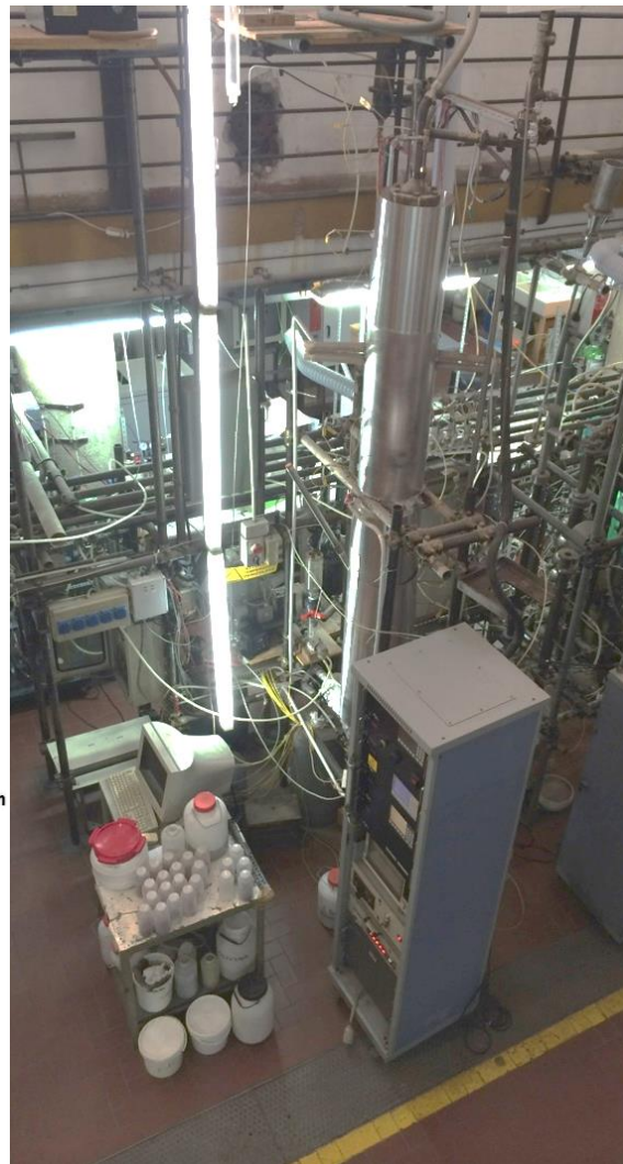
Figure 5-1 The 110 mm ID stainless steel fluidized bed combustor
