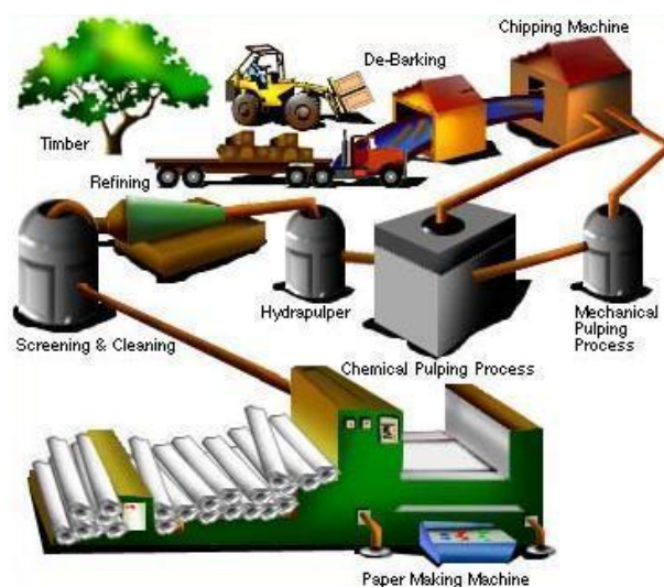
Figure 1-3 Paper production process (Source: Form Factory (Malaysia) Sdn Bhd.)
