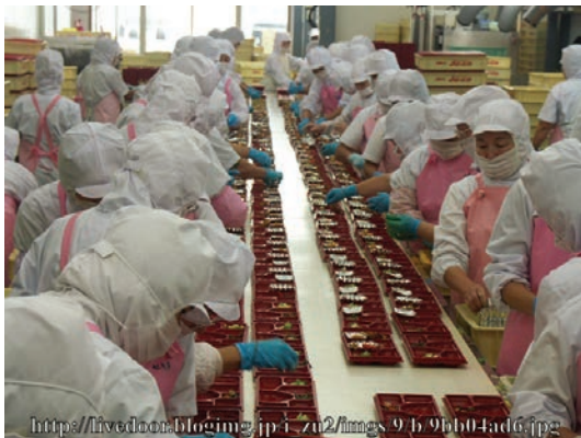
Fig.1 Line production in a lunch box factory placing foods in a serving dish.
