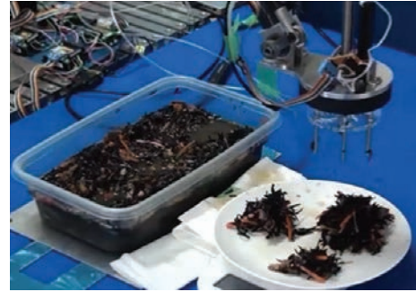
Fig.4 Controlling weight of the grasped food.
