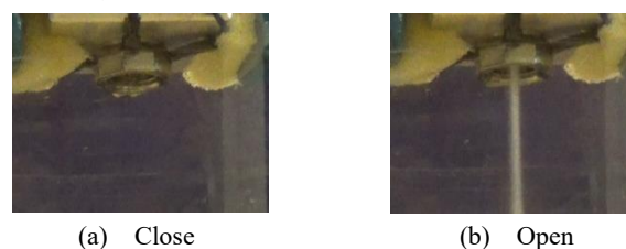
Fig. 6 Driving state of the control valve
