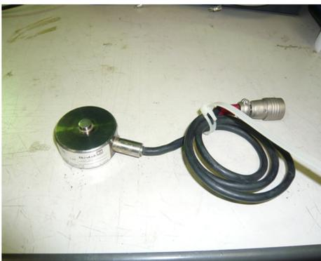
Figure 3.4.22 One-directional load cell.
