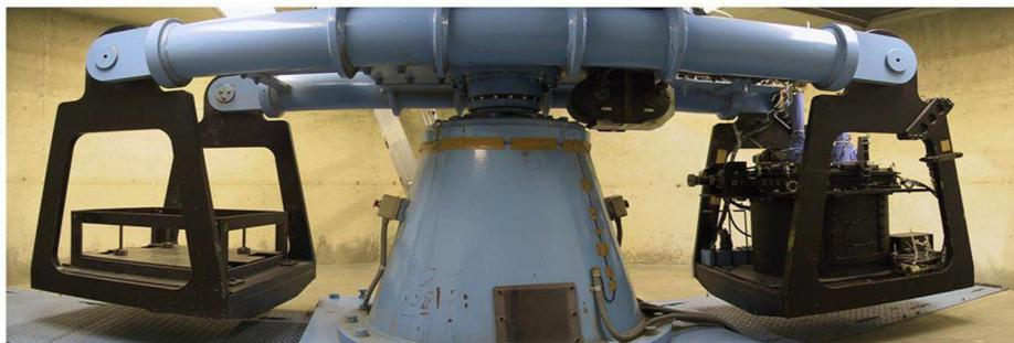
Figure 3.3.1 Tokyo Tech Mark III centrifuge.
