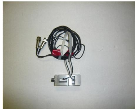
Figure 3.4.21 Two-directional load cell.
