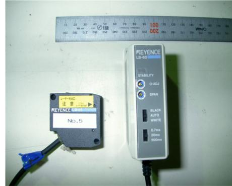
Figure 3.4.25 Laser displacement transducer.
