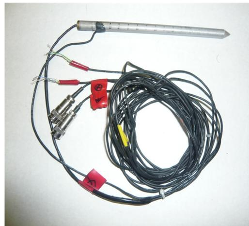
Figure 3.4.9 Picture of model pile.
