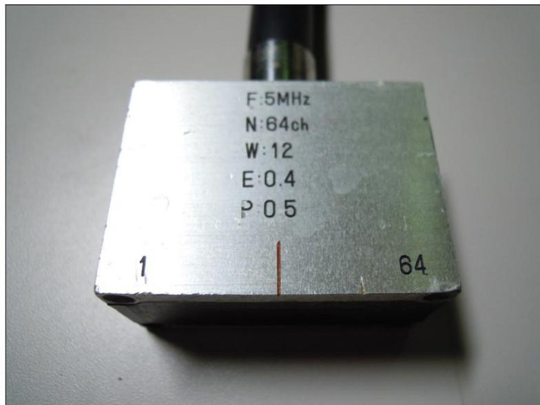
**Figure 3.1** 64 channels linear phased-array transducers.
