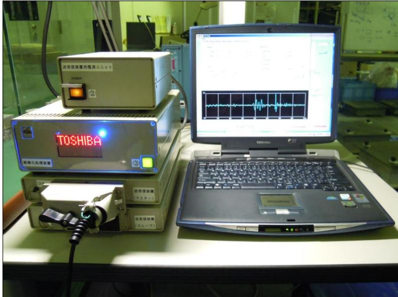
**Figure 3.2** Pulser-receiver and wave acquisition system.
