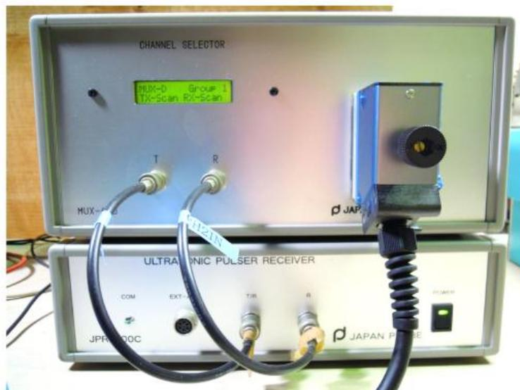
**Figure 4.2** Pulser-receiver system.
