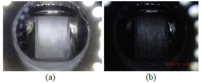
Fig.1 Photographs of the surface of liquid lithium film flows on the concaved wall in a high-vacuum ( < 10^{-3} \text{ Pa} ), i.e., at the saturation pressure of lithium, at the temperature : 220^\circ\text{C} , film thickness : h = 0.6 \text{ mm} , and flow velocity : U = 30 \text{ m/s} . Shutter speeds of the camera were (a) 1 ms and (b) 10 \mu\text{s} , respectively. These figures are quoted from Fig.7(a) and (b). in the paper experimented by Kobayashi, et. al. (9) .
