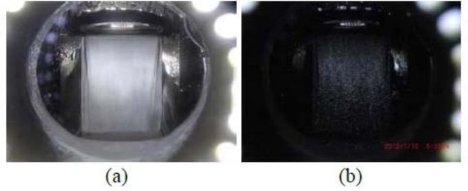
Fig.1 Photographs of the surface of liquid lithium film flows on the concaved wall in a high-vacuum ( $< 10^{-3} \text{ Pa}$ ), i.e., at the saturation pressure of lithium, at the temperature :  $220^\circ\text{C}$ , film thickness :  $h = 0.6 \text{ mm}$ , and flow velocity :  $U = 30 \text{ m/s}$ . Shutter speeds of the camera were (a) 1 ms and (b)  $10 \mu\text{s}$ , respectively. These figures are quoted from Fig.7(a) and (b). in the paper experimented by Kobayashi, et. al.<sup>(9)</sup>.
