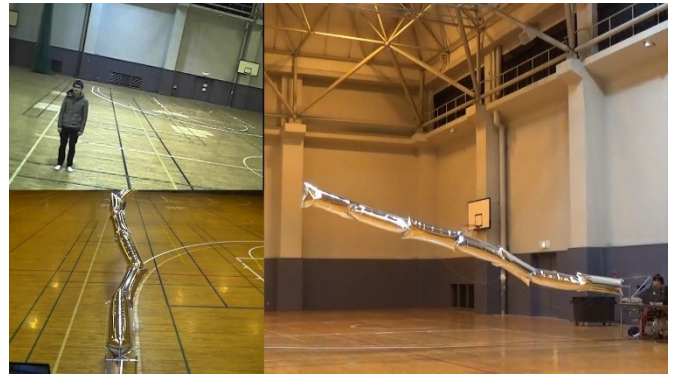
Fig. 6 Motion of the 7 link arm, 7 m long (upper left: a view from a camera mounted at the arm tip, lower-left: arm motion viewed from the robot base, right: whole view of the arm)
