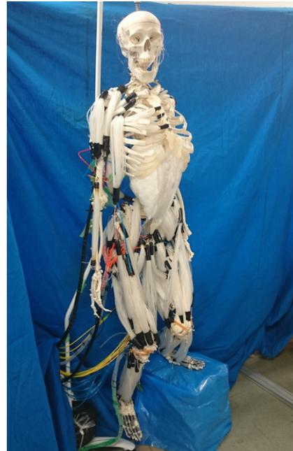
Fig.1 The musculoskeletal robot using multifilament pneumatic muscles
