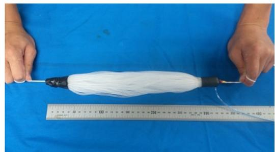
Fig.2 Multifilament pneumatic muscle (Air pressure 0.25MPa)
