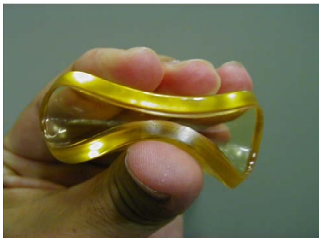
Photo 4-2 Cured resin of E-VBP2F with excellent flexibility and toughness
