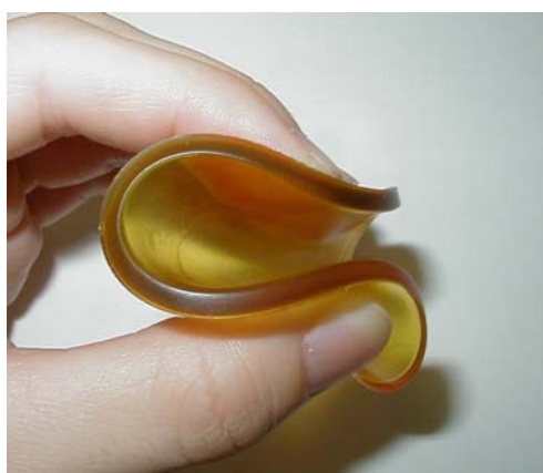
Photo 4-3 180 degree bending test result of E-VAL2F(a) cured resins
