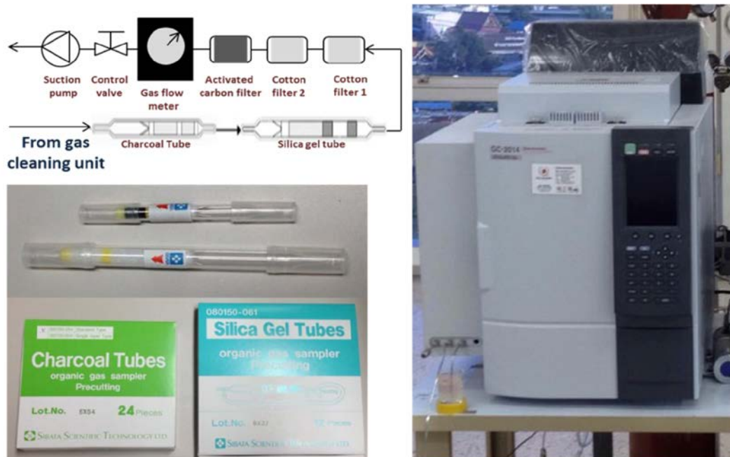
Figure 5.6: Schematic diagram of the dry sampling, the flow measurement method and the analysis facility
