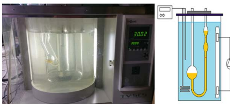
Figure 2.2: Experimental setup used to measure the viscosity of scrubbing fluids in the temperature range of 30°C-60°C by TV-SES Model, Thomas Kinetic Viscosity Bath
