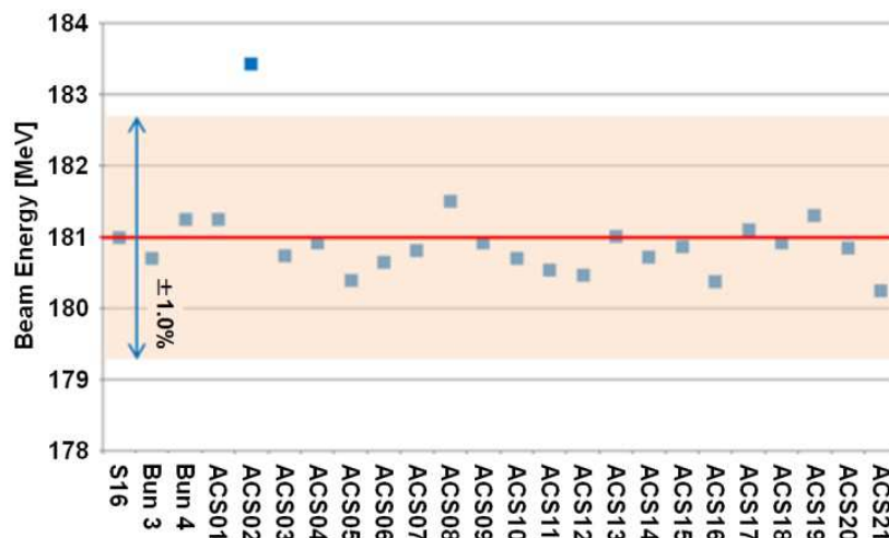
Figure 8-1: Beam energy data obtained by various FCT pairs at 181-MeV operation. S16 means the 16th SDTL cavity, Bun 3 and Bun 4 are the 1st and the 2nd Buncher cavity in MEBT2.
