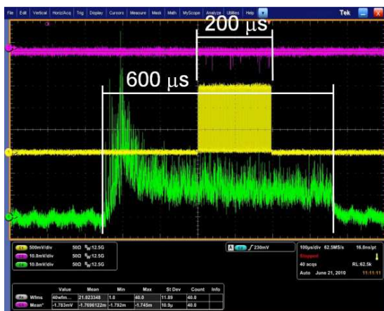
Figure 7-11: Signals from a gas proportional BLM (green) and scintillation BLM (magenta) at SDTL13. Time scale is 100 \mu s/div. The beam current signal from SCT is also shown (yellow).
