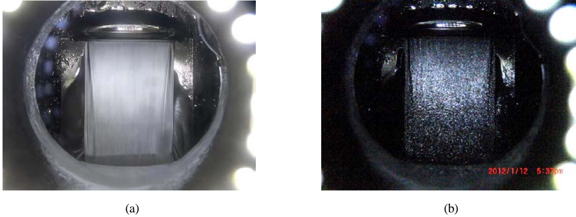
Fig.1 Photographs of the surface of liquid lithium film flows on the concave wall in a high-vacuum ( < 10^{-3} Pa), i. e., 220 °C in temperature at the saturation pressure of lithium, h = 0.6 mm in thickness, and U = 30 m/s in velocity. Strobe exposures of camera were (a) 1 ms and (b) 10 \mu s, respectively. These figures are quoted Fig.7 (a) and (b) in the paper experimented by Kobayashi, et al. (8) .
