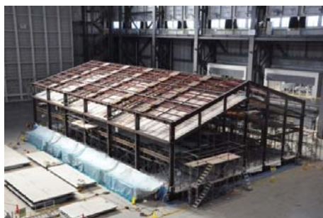
Photo 2 Full-scale Gymnasium Specimen
