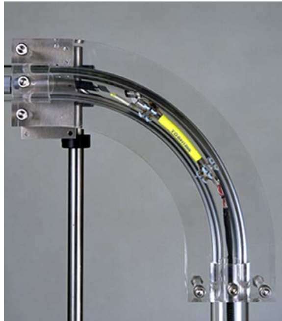
Fig.7.25 Locomotion through a vertical elbow-joint
