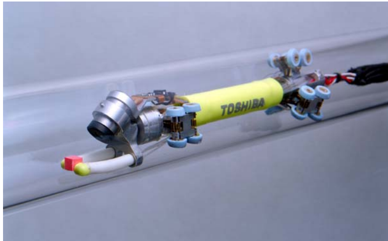
Fig.7.27 Collection of the small object in 1-inch pipes
