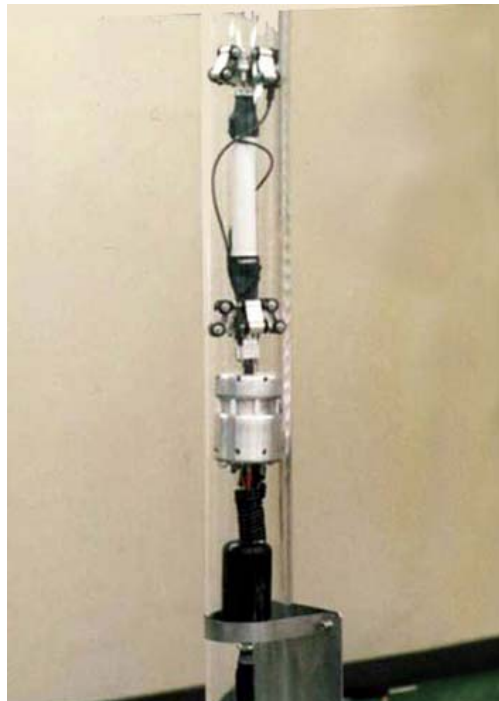
Fig.2.10 Photograph of the in-pipe mobile robot for 3-inch pipes (50),(51)
