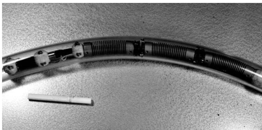
Fig. 1.6 An in-pipe mobile robot for 1-inch pipes by Hayashi (35)
