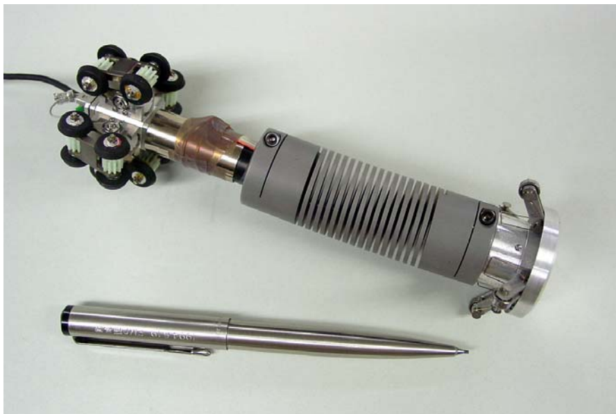
Fig.4.4 Photograph of the in-pipe mobile robot for bent pipes
