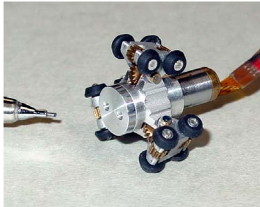
Fig.2.7 Photograph of the wheel drive mechanism for 1-inch pipes (49)
