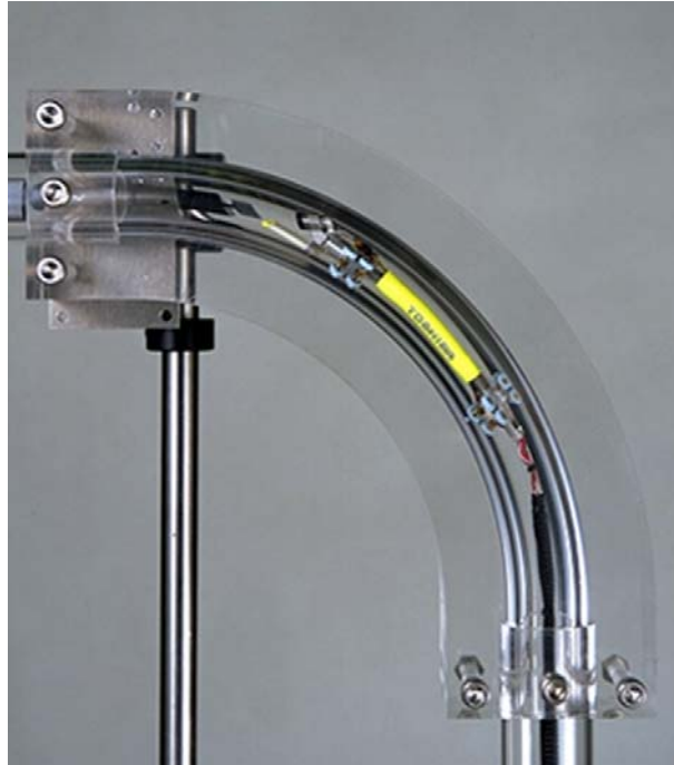
Fig.2.9 Photograph of the in-pipe mobile robot for 1-inch pipes (49)
