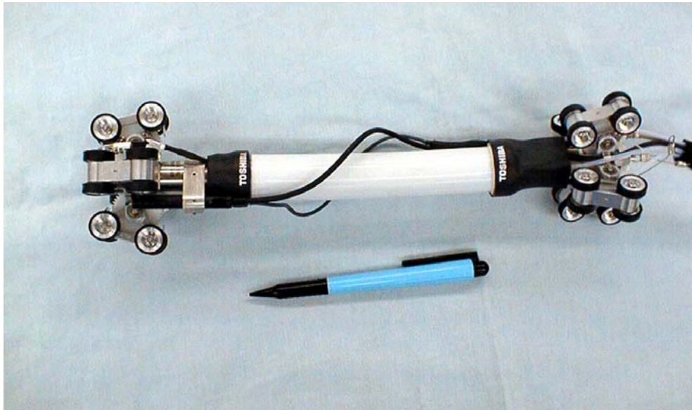
Fig.7.31 Photograph of in-pipe mobile robot for 3-inch pipes
