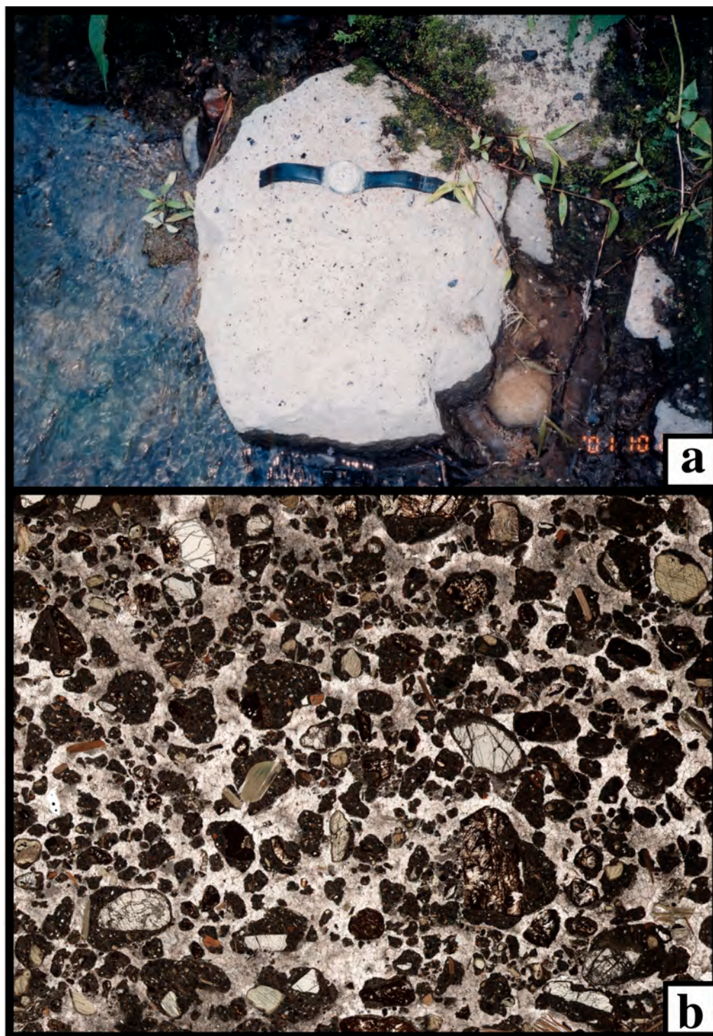
Fig. 2-3. a: the photograph of alnöite outcrop located along the Auluta river. b: thin section photomicrograph of the alnöite which displays two-separated zone representing well-crystallized calcite matrix (white) including rounded glassy zone (black). Horizontal axis of the flame = 3 cm.
