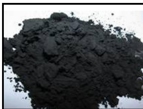
Fig. 2.4 The appearance of vanadate glass powder.
