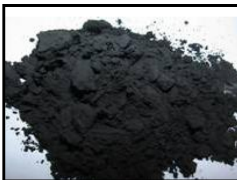
Fig. 2.4 The appearance of vanadate glass powder.
