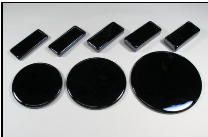
Fig. 2.3 The appearance of vanadate glass blocks.
