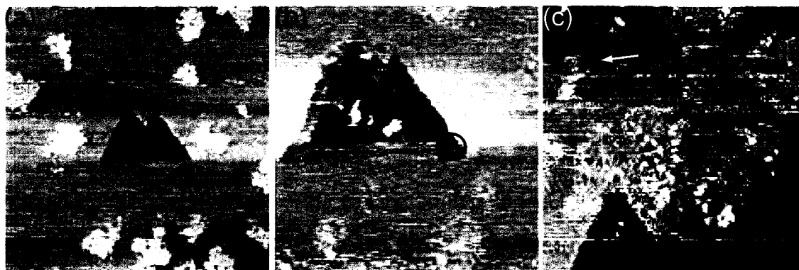
Fig. 6.4. Change of STM image contrast with redosing \text{O}_2 to the oxidized surface. The partially oxidized surface shown in Fig. 6.2 (b) was exposed to the \text{O}_2 at 1.6 \times 10^{-4} \text{ Pa} at room temperature for 4 min. (a) Terrace and added oxide islands before redosing \text{O}_2 ( 500 \times 500 \text{ \AA}^2 , V=500 \text{ mV} , I=0.05 \text{ nA} ). (b) Indistinct light patches almost in the same place as in (a) just after redosing \text{O}_2 ( 300 \times 300 \text{ \AA}^2 , V=500 \text{ mV} , I=0.05 \text{ nA} ). A kink has formed in the terrace island edge as the surrounding Cu terrace is etched. (c) Distinct light patches in the same place as (a) and (b) after evacuation of \text{O}_2 ( 300 \times 300 \text{ \AA}^2 , V=500 \text{ mV} , I=0.05 \text{ nA} ). The kink in Fig. 6 (b) has moved along the step in the direction of the arrow, i.e. \langle 01\bar{1} \rangle .
