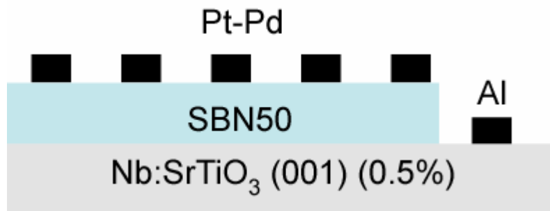
Fig. I-4 Schematic drawing of setting for current (I) – voltage (V) measurements and capacitance measurements. Al electrodes were used for Nb:STO (Nb=0.5%) contact and Pt-Pd electrodes were used for SBN 50 films contact.
